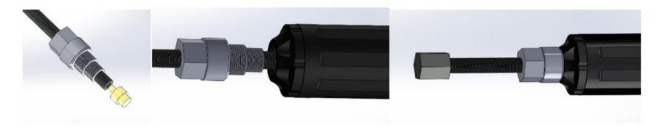
Grease and then insert .30 cal or .223 brass piece depending on suppressor size.
